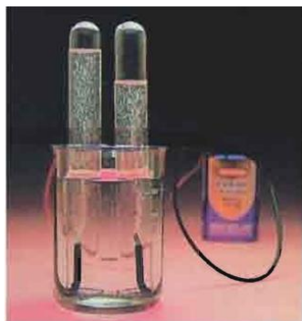
Electrolysis of Water In electrolysis of water, hydrogen (at right) and oxygen (at left) gases are produced in 2:1 ratio.
